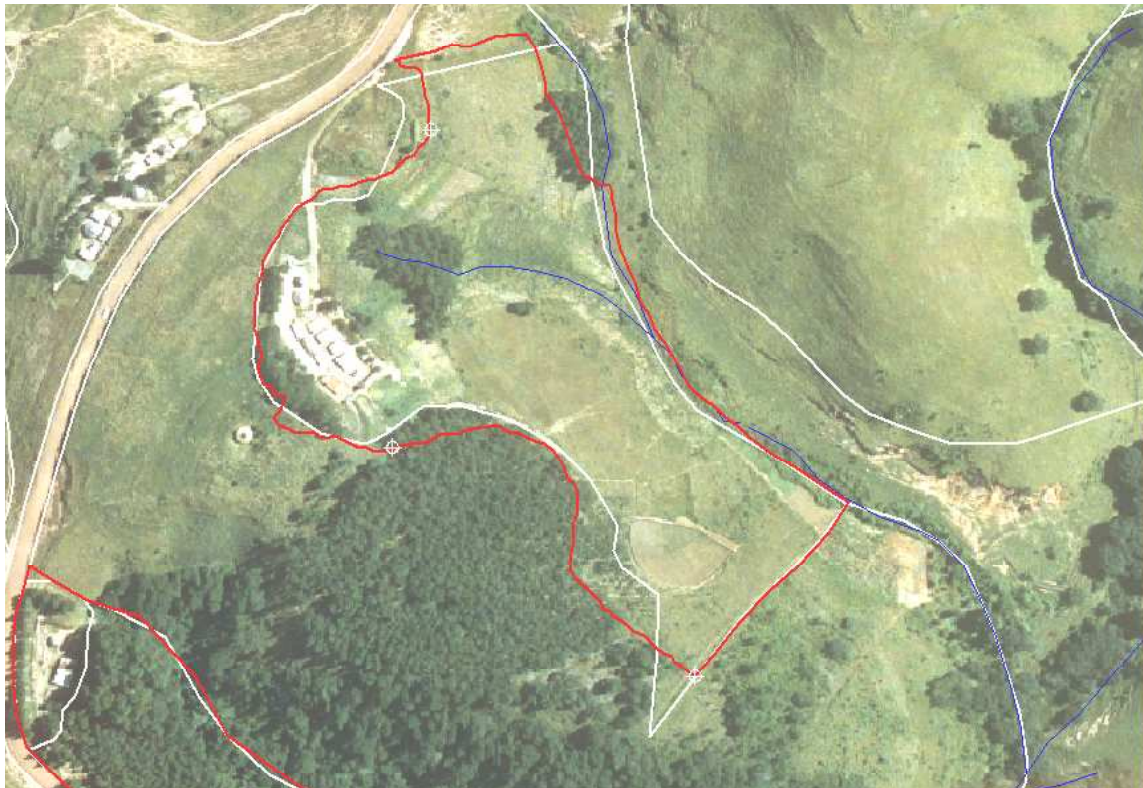
Figure 4 Nsele family land right boundary as demarcated by aerial photo interpretation (white line) compared with the GPS walk trail (red line). Note the boundary pegs along the GPS trail as pointed out by the Induna and logged in GPS.
