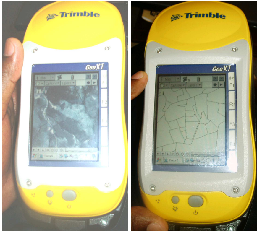
Figure 2 A high accuracy hand-held GPS unit displaying rectified aerial photo as a background image map (left) and a vector map (right)
