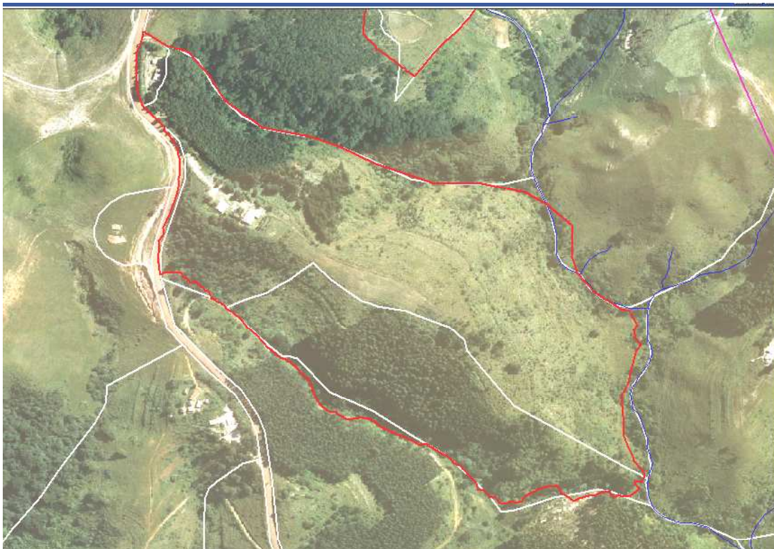
Figure 3 Nxumalo brothers outer boundary as demarcated using aerial photo interpretation (white) compared with a GPS walk-trail (red). Note that the boundary is mainly within the stream channel where walking as not possible.
